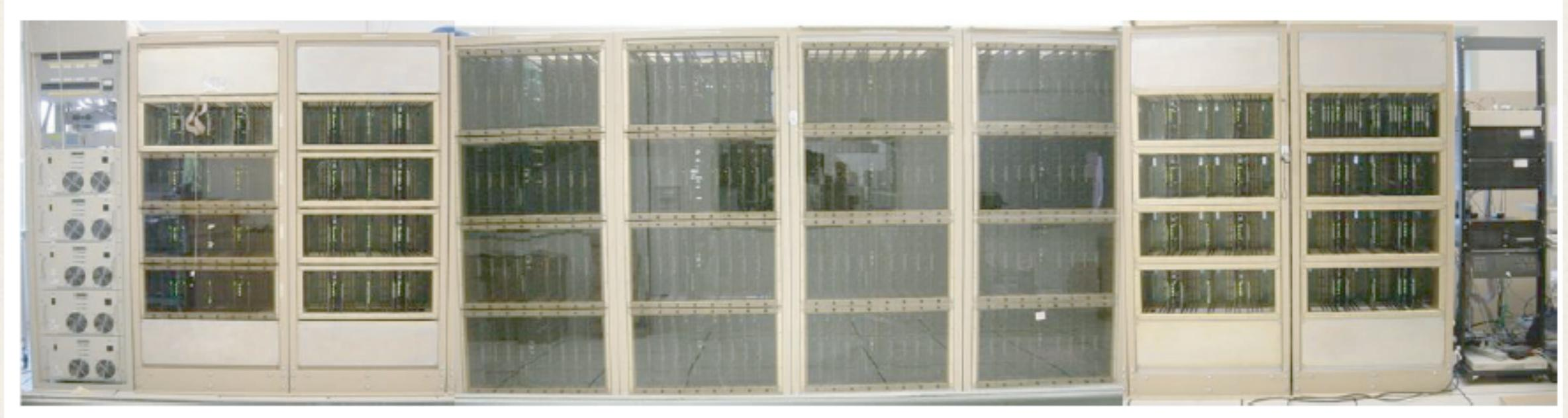
From left to right: Power supply, station racks, correlator racks, station racks, computer.
